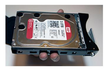
The HDD enclosures can hold 3.5" or 2.5" disks and are quite sturdy, with rubber pads
